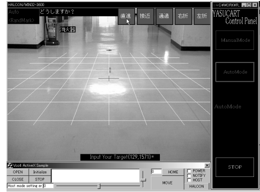
Fig. 3: Example of touch panel display for the interactive user interface
