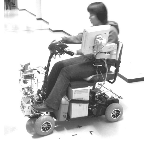
Fig. 6: Electric cart with the developed auto-driving system
