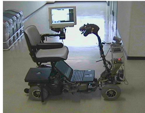
Fig. 7. Welfare electric cart with the auto-driving system.
