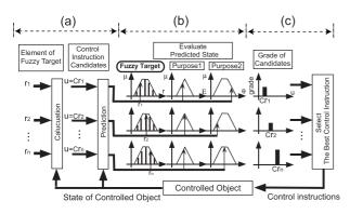
Fig. 3 An intelligent controller based on fuzzy target.
