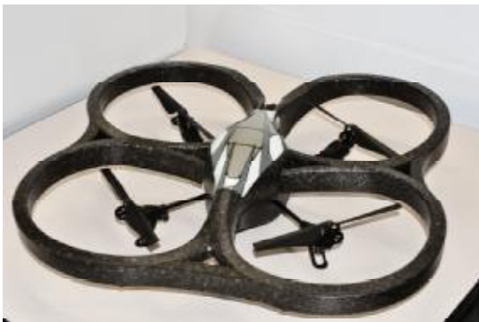
Fig. 1 A rotorcraft UAV propelled by four rotors.
